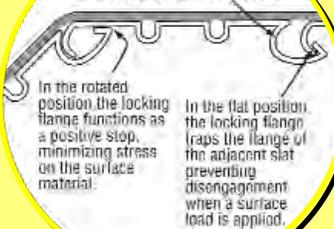
In the rotated position the locking flange functions as a positive stop, minimizing stress on the surface material.
