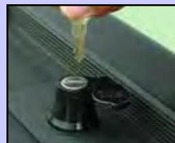
For the colder regions, we have developed a key slot cover to prevent water from entering the lock mechanism and freezing.
